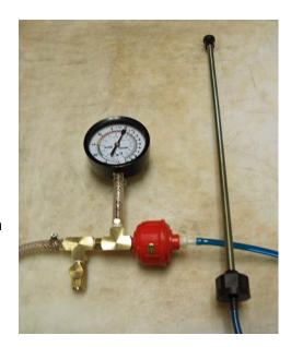
All brass parts have been wrapped with Teflon tape before being screwed together. Hose barbs to hose assemblies should be strengthened with the addition of a hose clamp.
