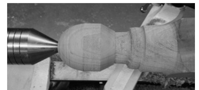
Drilled, laid out, and partially turned
