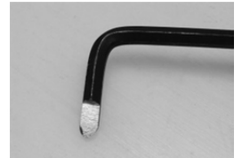
Tool tip ground to shape
