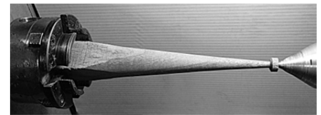
Round then taper the blank
