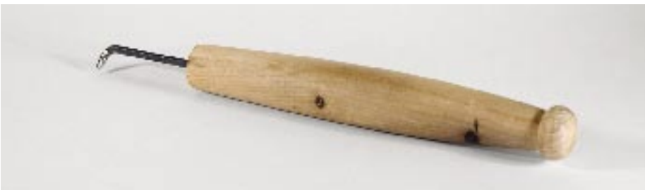
This homemade "finger saver" will help you hold segmented pieces in place and safely retrieve them. The steel is made from a discarded Allen wrench modified with a ground tip.
