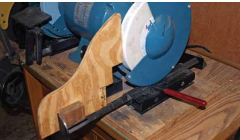
Using a simple shopmade jig to set up your sharpening jig for repeatable distances saves time and tool wear.
